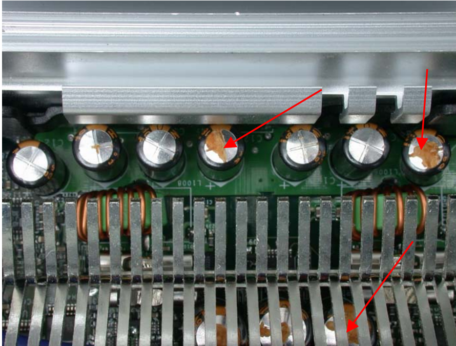
Figure 1 - The consequences of running a computer above its rated temperature
